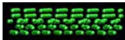
Fig.3: Atomic configuration of “TB region” near (001) \Sigma 5 GB of Si after relaxation by hybrid classical/TB-MD method.
