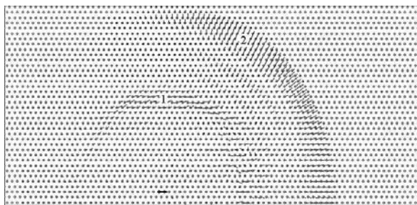
Fig.1. The picture of the atomic displacements in two-dimensional Al at the moment of time 1.5 ps relatively to the beginning of the experiment (the scale 30:1). The value of the initial velocity is equal to 3000 m/s. The cross waves – 1, the longitudinal waves – 2. The place and the direction of the initial impulse are marked by the arrow. The picture of atomic displacements is symmetric relatively the direction of the initial impulse.
